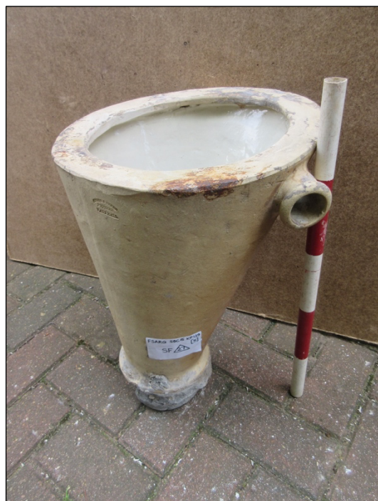
Fig 8a: According to the catalogue (Fig 8b) this is an 'improved conical deep pattern Hopper and Trap'.
